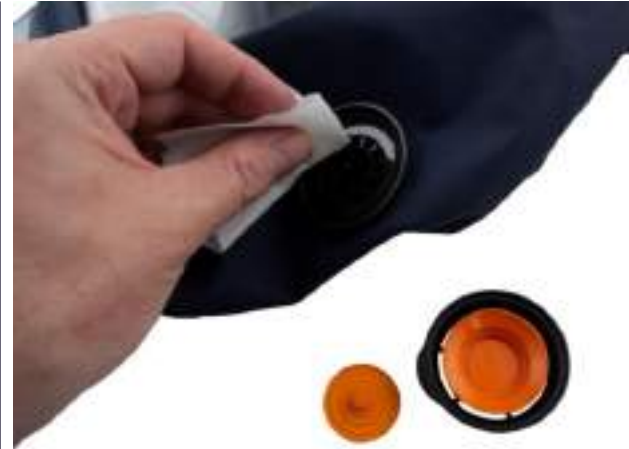
6.5 Clean the valve seat and check that the valve seat is ok.
